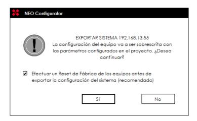
By default, the Export will perform a **factory reset** of NEO devices before transmitting the project configuration. In this dialog box, you can disable the initial factory reset. To do this, you must uncheck the checkbox that is shown and that will be marked by default. The factory reset of the devices is recommended to start the export on a clean system, with factory parameters and initial states. The factory reset is performed while preserving the network configuration of the devices.
