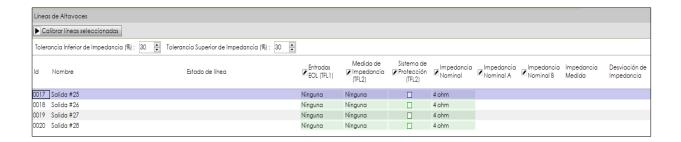
**NOTE:** Settings for speaker line monitoring are stored on Extension devices. The System Controller only saves settings for monitoring its own speaker lines.
