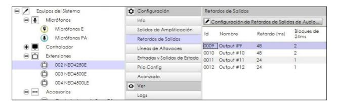
Delays are applied to outputs in **blocks of 24 milliseconds**, up to a **maximum of 6 blocks or 144 milliseconds**. It is not essential that the entire 24 milliseconds of each block be used, but it should be borne in mind that the milliseconds that remain unused in one block cannot be used in another output delay.
