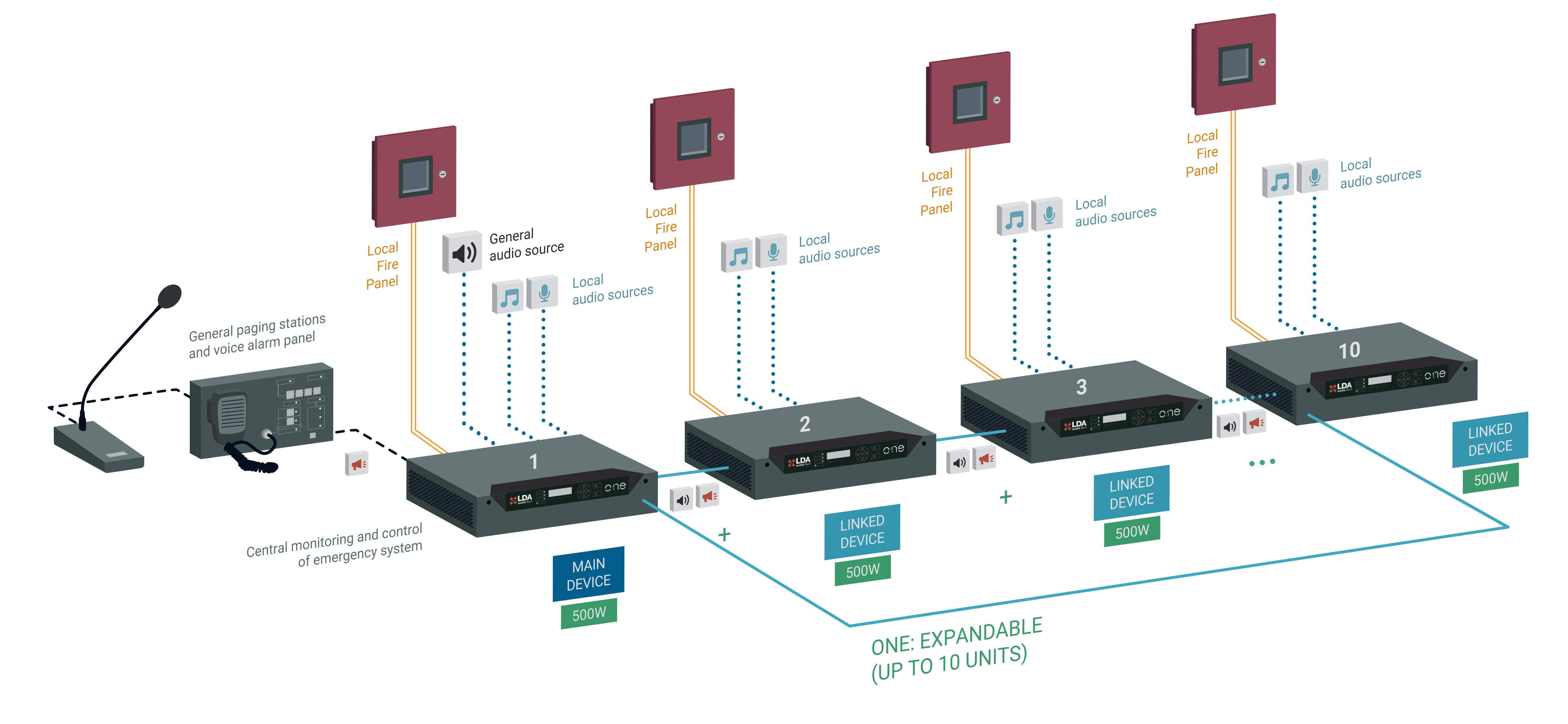
• • • • • • Analogue audio – – – LDA ACSI® paging station bus (UTP cable) **UTP** Cable Fire alarm local zones and Fire alarm general / reset
