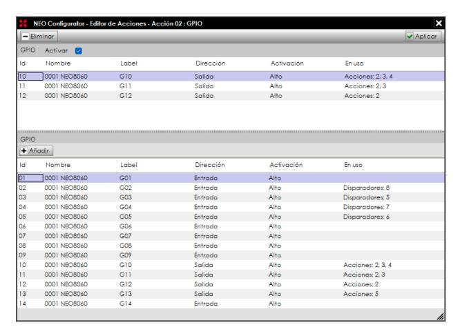
The bottom pane displays the list of system GPIO ports, from which you can select one or more ports and add them to the action using the "Add" button. The top panel shows the ports already added to the action. With the "Delete" button, remove the ports you want from the top panel by selecting them previously. Checking the "Enable" box indicates that the action will activate the selected ports, if you want the action to do is to disable them, you will have to uncheck that box.
