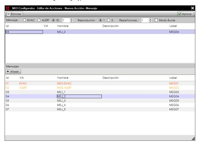
The controls in the top panel define which message the action will play and how it will be done. These controls are divided into three sections:
