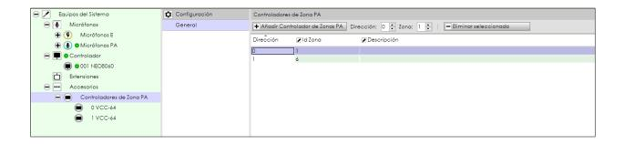
**NOTE:** The Configuration Filter **General** for PA zone controllers will only be displayed with user profile **Installer** or **Maintainer** (See **2.4.3. Users**)
