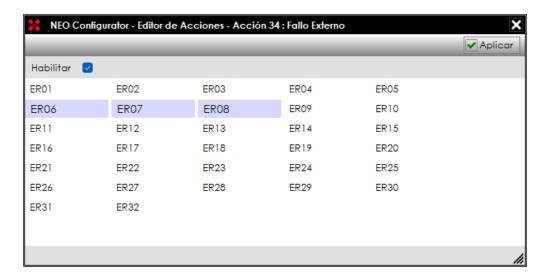
In the **middle** panel of the window, the **32 possible errors** that we can enable or disable are displayed. To select an error, simply **click** on it. Holding down the **Ctrl key** will allow you **to add other errors to the selection or remove them** if they are already selected.
