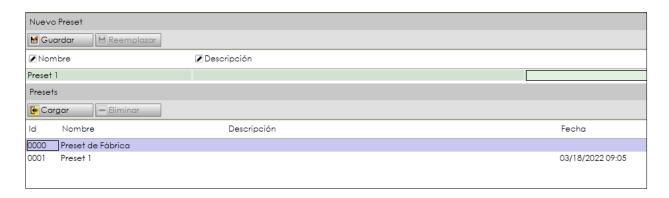
To reconfigure the system with the parameters stored in a preset, simply select it from the list in the "**Presets**" panel and then click on "**Load**".
