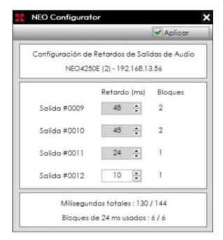
At the bottom of the window, the total milliseconds used in the delays are displayed, as well as the total 24-millisecond blocks used.
