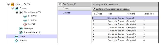
Groups are entities designed to provide greater flexibility and capacity to address the buttons of ACSI devices, both VA microphones and PA microphones. See 4.1.2. c. ACSI Device Button Configuration
