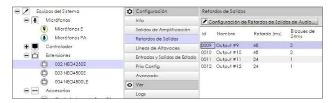
Delays are applied to outputs in **blocks of 24 milliseconds**, up to a **maximum of 6 blocks or 144 milliseconds**. It is not essential that the entire 24 milliseconds of each block be used, but it should be borne in mind that the milliseconds that remain unused in one block cannot be used in another output delay.
