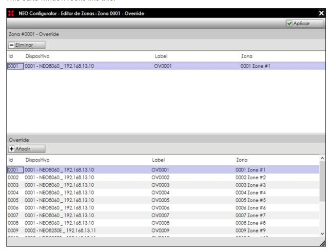
The upper panel shows the list of override departures currently assigned to the area, while the lower panel will have the list with all the override outputs of the system.
