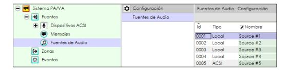
Selecting the configuration filter will display the list of sources. Only the **Id, Type** and **Name parameters** of the sources will be displayed, with only the latter being editable.
