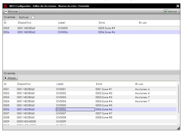
The bottom panel displays the list of the system's **Override** ports. You can select one or more and add them to the action using the "**Add**" button. The top panel shows the ports already added to the action. With the "**Delete**" button, you can remove already added ports by selecting them in advance in the top panel. You will have to check the "**Enable**" box if you want the action to activate the selected ports or uncheck it otherwise.
