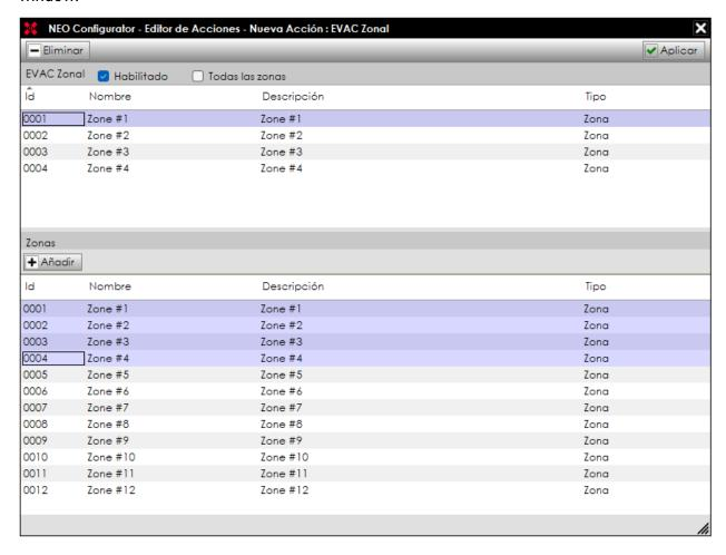
Checking the "Enabled" box will cause the evacuation message to play in the selected areas. Unchecking the "Enabled" box will stop the playback of the evacuation message in the selected areas, if applicable.
