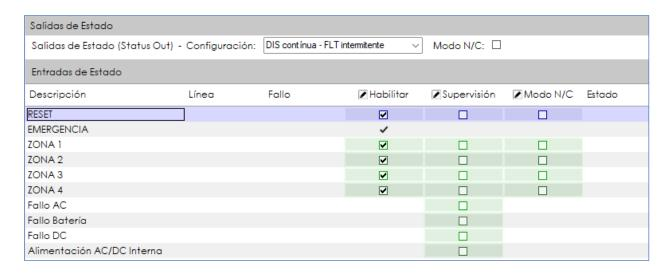
In an Extension we can only configure the Status Out and Status Input (Reset, Emergency and Areas), Batt Charger (AC Fault, Battery Fault and DC Fault) and Internal AC/DC Power. For a detailed explanation of monitoring and configuring these parameters, see 4.1.4. h. Controller: Instate inputs and outputs
