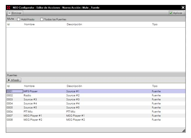
This time instead of a numeric field to specify a volume value, we will have the "**Enabled**" box that will determine when checking or unchecking it if what you want is to enable or disable muting.
