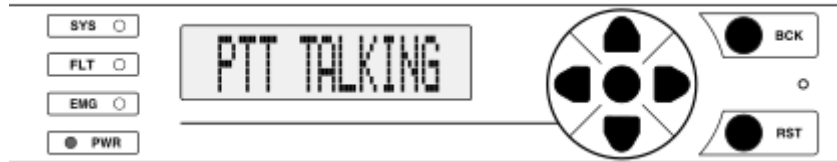
Figure 23: View of the PTT status info on the LCD display
