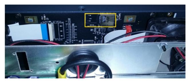
This card is find in the device's front side, just behind the touchscreen. In the front card is where all regarding PA messages is stored. This card must have a 2GB format using FAT16 filesystem and be the primary partition.
