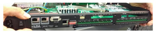
If the microprocessor board is lifted or incorrectly embedded, put it carefully again inside the socket below the CobraNet board. If you need it you can remove the upper part of the case, pull off the CobraNet board, place the microprocessor board in the socket and put again the CobraNet board.
