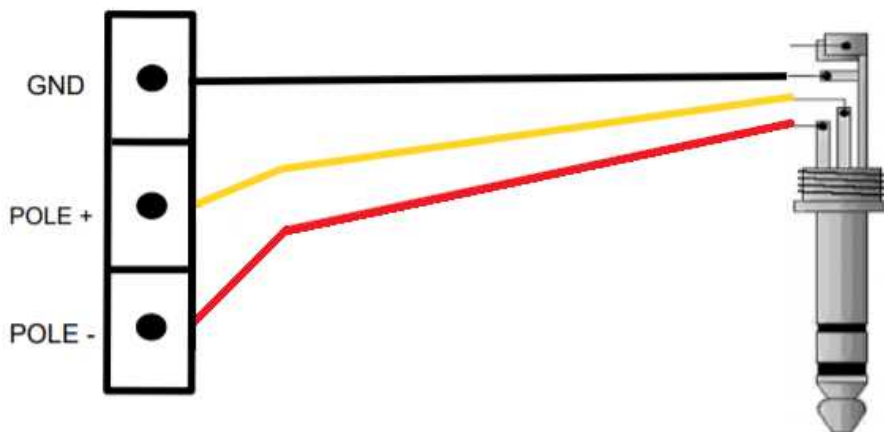
Diagram 3: Balanced audio output connection to Jack
