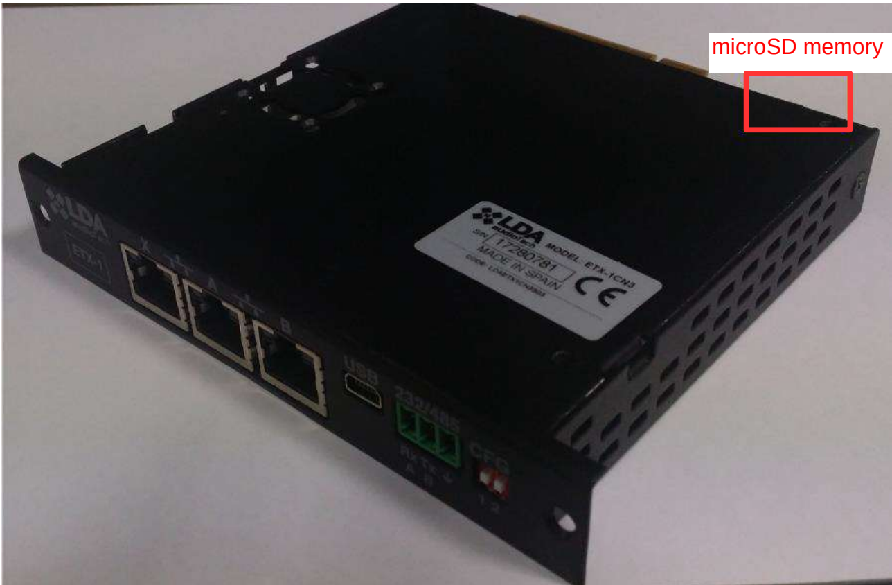
Picture 3: microSD card on ETX module
