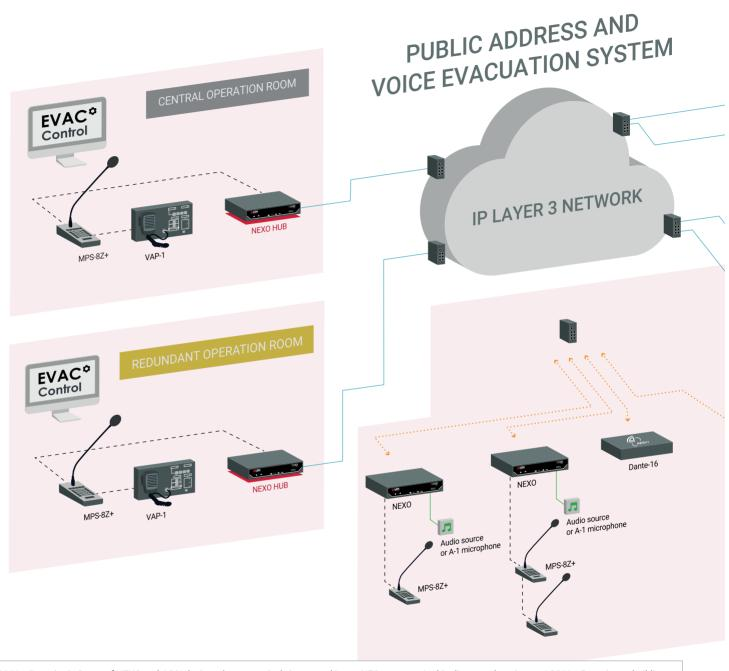
ACSINet Domain → Group of NEXO and ACSI devices that are natively integrated into a NEO+ system. In this diagram, there is one ACSINet Domain per building. ACSINet Cluster → Group of NEXO Hub and ACSI equipment forming a multisite structure. This diagram features a total of one ACSINet Cluster.
