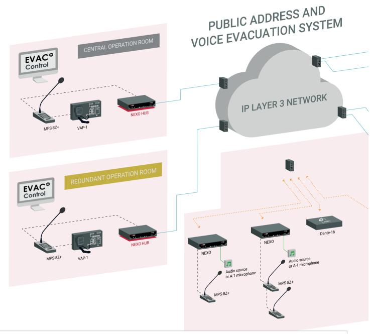
ACSINet Domain → Group of NEXO and ACSI devices that are natively integrated into a NEO+ system. In this diagram, there is one ACSINet Domain per building.
