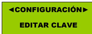
Once the new code is requested, it is introduced using the number buttons on the front panel and the OK key is pressed; a confirmation will be requested, and the code must be written again.
