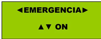
The emergency status priority to occupy the channel is as follows: first voice messages broadcast by the microphones, and then the evacuation sequence. Therefore, if there is an evacuation sequence or if it is being broadcast and a microphone wants the floor, the equipment will switch to the microphone, and after the microphone has finished speaking it will switch back to the emergency sequence.
