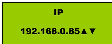
The last number of the IP address can be changed with the keyboard, using the up/down arrow keys. The level of increase is one by one, and it is also cyclic, which means you can go from the maximum value to the minimum one in just one step.
