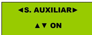
If in this status any of the two microphone inputs (inputs 6 and 7) are configured as CD input, it will be given way. If a microphone that has more priority than the CD input requests the floor, the CD input will switch and give the floor to the microphone. Once that microphone has finished talking, the equipment will switch back to the CD input.
